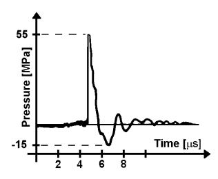
Fig. 2. Pressure profile obtained with a PVDF needle hydrophone positioned at the *F*2 focus of the electrohydraulic shock wave generator.
